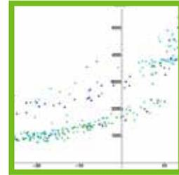
**Energy use (kWh) on days with similar temperatures:** A tight curve indicates a well-controlled building utilizing energy optimization. A scattered curve illustrates a lack of consistency.
